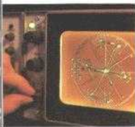
Chrome vector scope at Southern Satellite Systems indicating color saturation of Torus transmission.
